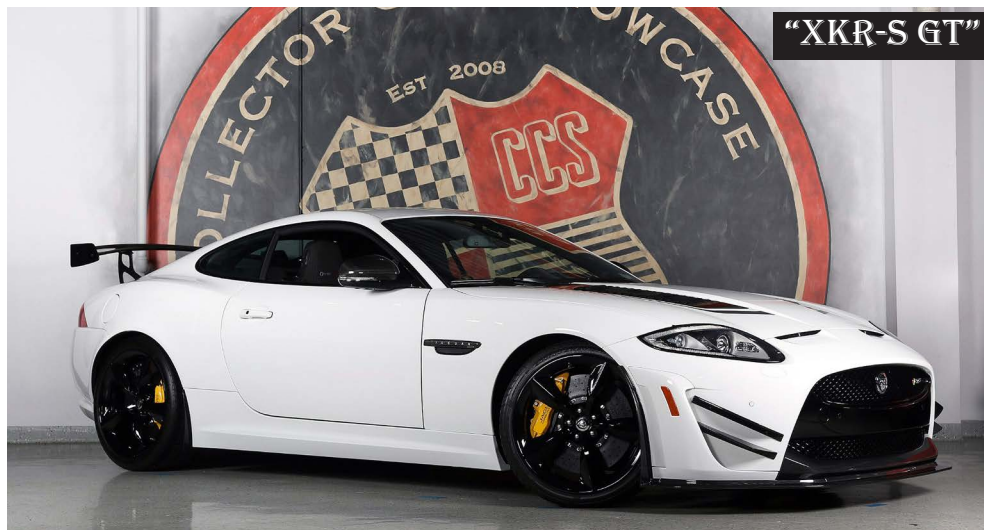
2013 "XKR-S GT" was a 300km/hour up-rated version of XKR-S coupé with a worldwide production of 45 units. The GT included a host of upgrades including a wider front track, stiffer suspension, carbon ceramic brakes and a reduction in kerbweight.
