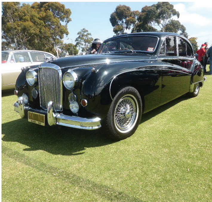
A late Mark VII fitted with non- standard wire wheels.
