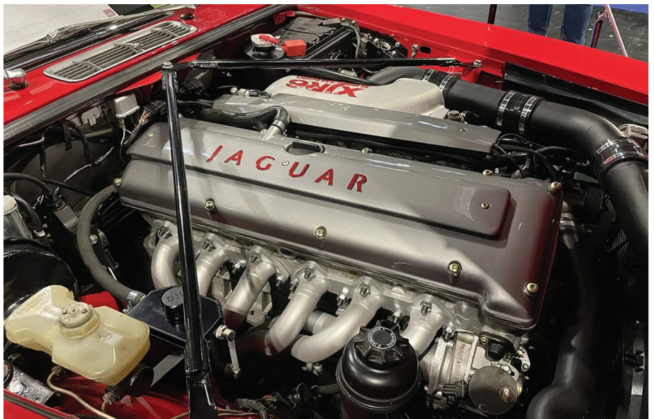
This XJ-C is now powered by a 4.0-litre supercharged AJ16 from an X300 XJR
