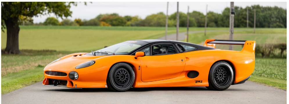
TWR developed six road cars called the XJ220-S, featuring one-piece carbon-fibre-reinforced polymer front and rear bodywork; the engine was tuned to 690 hp).
