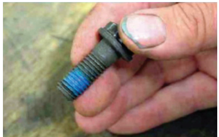
Some bolts come with the thread-lock already applied.
