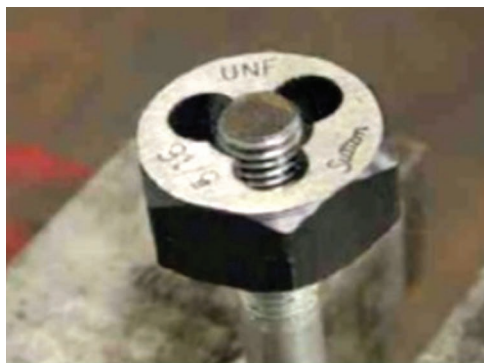
Using die nuts to clean threads should be avoided if possible as they weaken the bolt.
