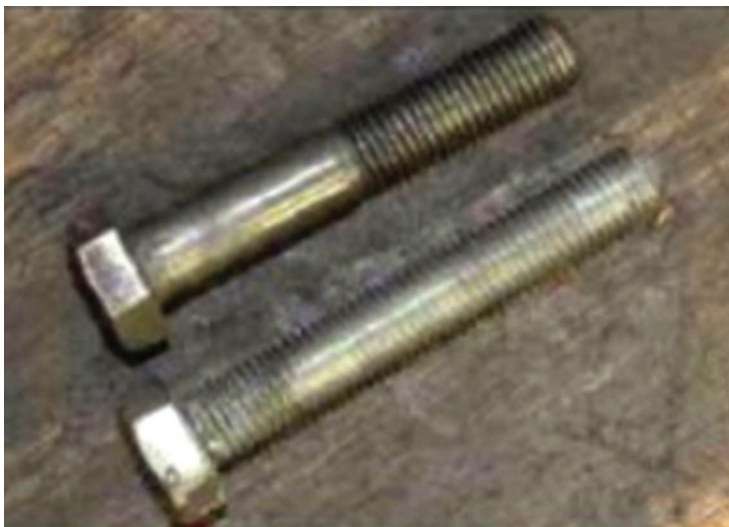
Thread length will usually be kept as short as possible to maintain strength.
