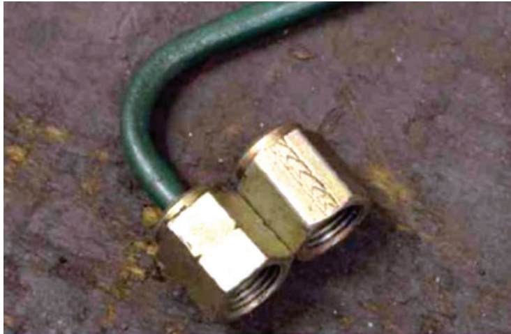
The metric female union can have identifying notches or a band of Ms - or nothing.
