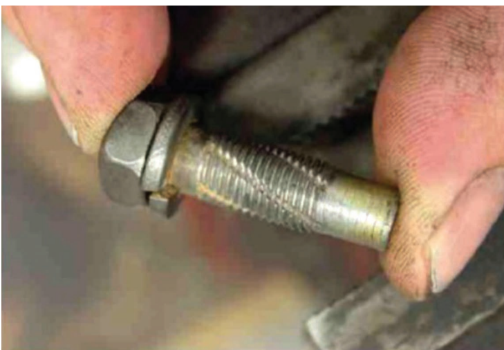
This suspension bolt is slotted as a self cleaning aid.
