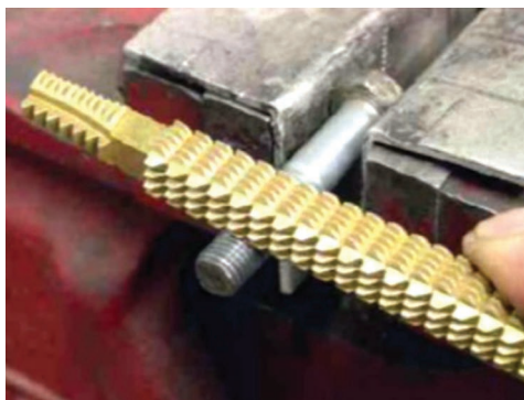
A thread file is a much better option if you need to remove individual burrs.
