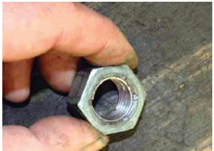
Some nuts come with a Heli-coil already installed for added durability.
