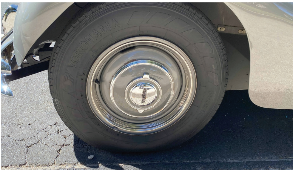
From 1953, the 16 inch rim width increased from 5 to 5½ inches
