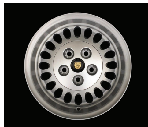
Metric 390 x 180 TD35 "Teardrop" rim fitted to XJ40 Sovereign and Daimler from 1986 to 1992
