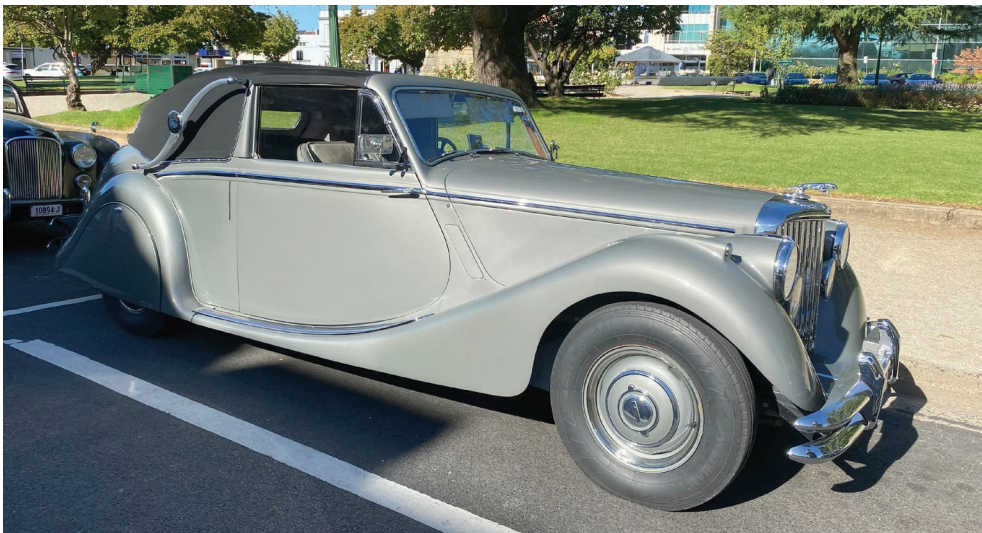
The first Jaguars with bolt-on wheels were the Mark V and XK 120.
