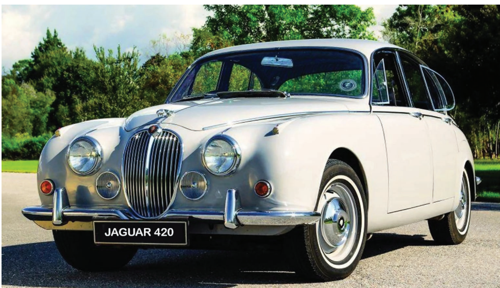
The Mark 1 and early Mark 2s had 4½ x 15 inch wheels, but the later cars up, to the 240 (shown above), had 5 x 15 inch rims.
