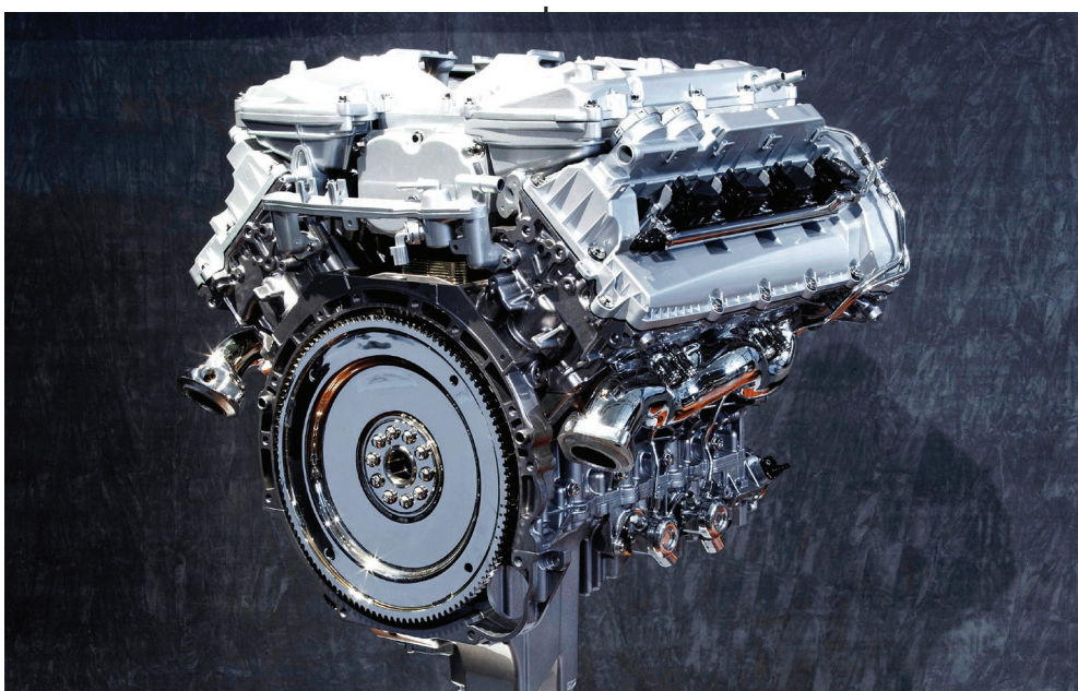
The Jaguar F-Type supercharged V-8 is used as a third engine to drive an oxidizer pump that feeds liquid-propellant to the rocket engine.
