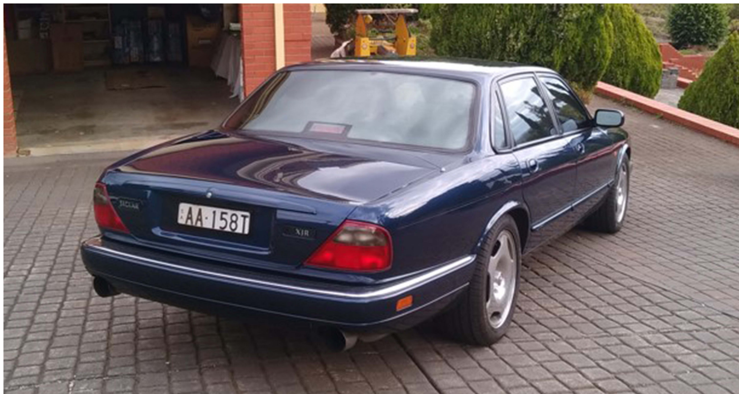
The rear of the XJR can be identified by the body-coloured boot-lid plinth, larger exhaust outlets, rear boot badge and special five-spoke "Sport" alloy wheels. The X300 XJR model is sometimes referred to as the "XJR6" to differentiate it from the later V8-engined X308 XJR.
