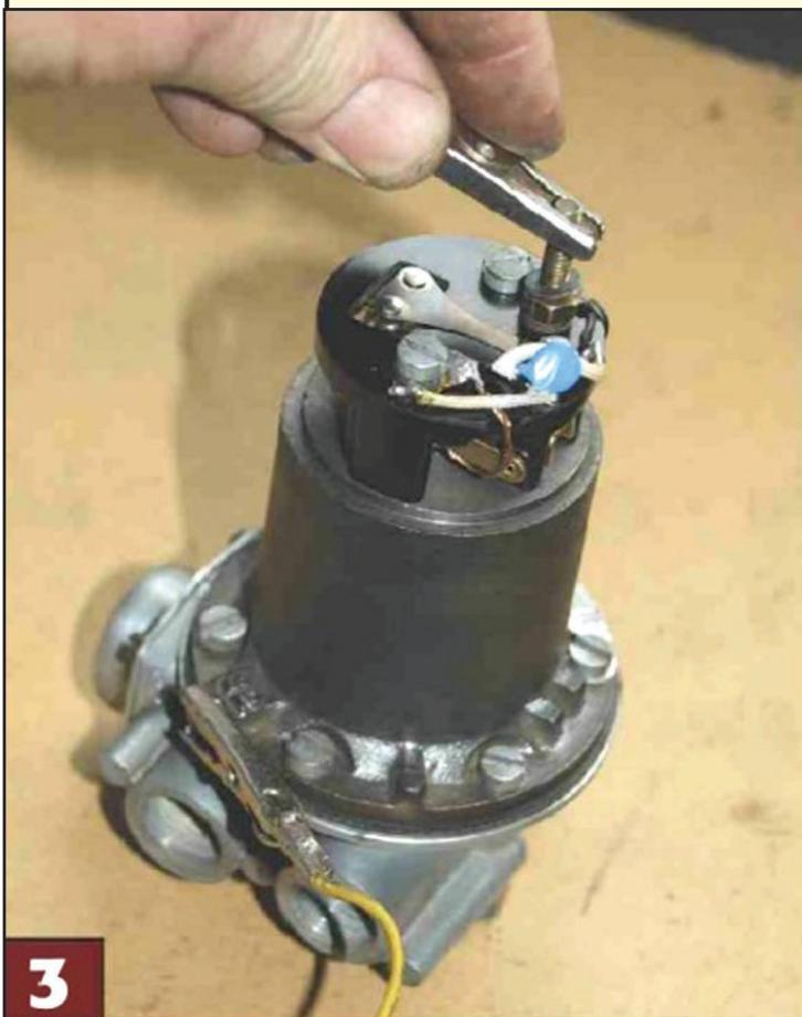
Check the pump for operation by attaching a 12-volt feed wire to the terminal stud and an earth to the body. Make sure the polarity is checked. In this case it is negative to earth.
