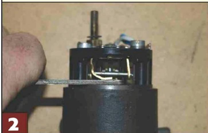
To adjust the rocker mechanism, insert feeler gauges to the value of 0.090in (2.3mm) between the top deck of the coil housing and the adjuster tag on the rocker mechanism. To adjust, simply move the tag in the appropriate direction. Be sure to recheck both measurements carefully afterwards.
