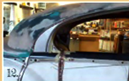
...and again, with the window runners removed, the rear doors were narrowed by 110mm and welded into place. Note the steel filler pieces added to improve the roof's rear quarter profile
