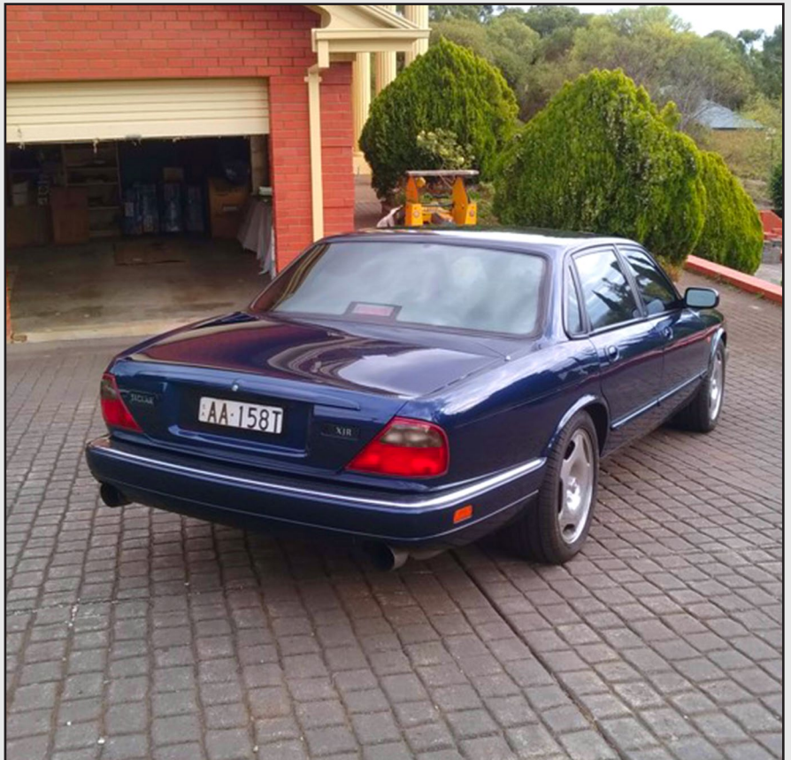
The rear of the XJR can be identified by the body-coloured boot-lid plinth, larger exhaust outlets, rear boot badge and special five-spoke "Sport" alloy wheels. The X300 XJR model is sometimes referred to as the "XJR6" to differentiate it from the later V8-engined X308 XJR.
