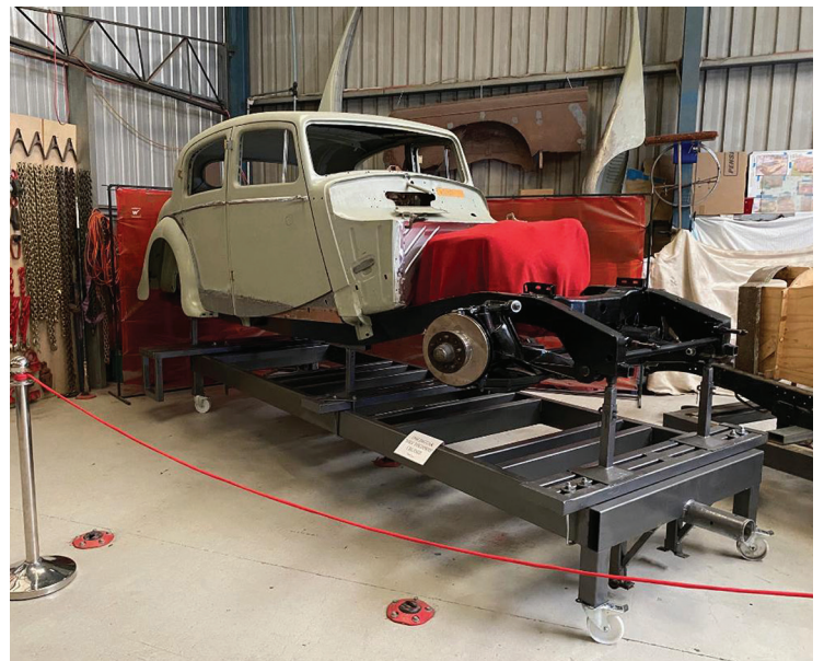
A Jaguar Mk V being upgraded and modified with a V8 engine
