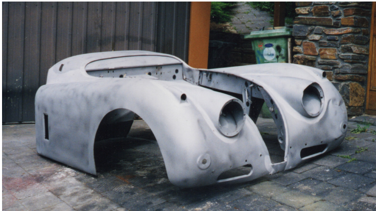
The body was taken back to bare metal, primed and reassembled onto the chassis. Work then started on the interior
