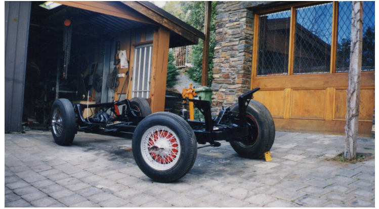
The chassis was taken back to bare metal, primed and painted, while the suspension and steering (converted to RHD) were refurbished
