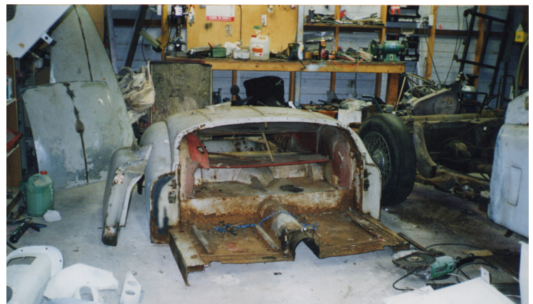
The body was removed from the chassis and then cut in half for ease of restoration
