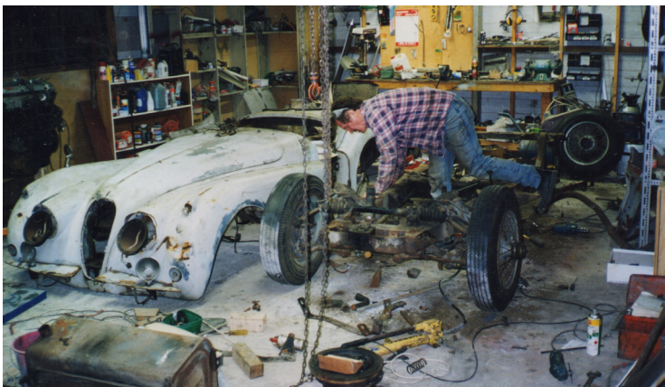
The body was removed from the chassis and then cut in half for ease of restoration
