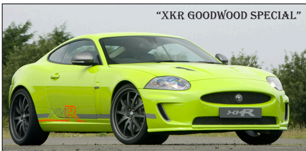
The XKR 'Goodwood Special' was a prototype designed to allow Jaguar's engineering team to extend performance boundaries. Fitted with 21-inch wheels and a lowered ride-height. The XKR had a one-off lime green paint scheme with satin graphite detailing.
