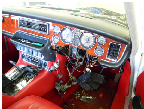
A "simple replacement" of steering column bearings which were shot!!!.
