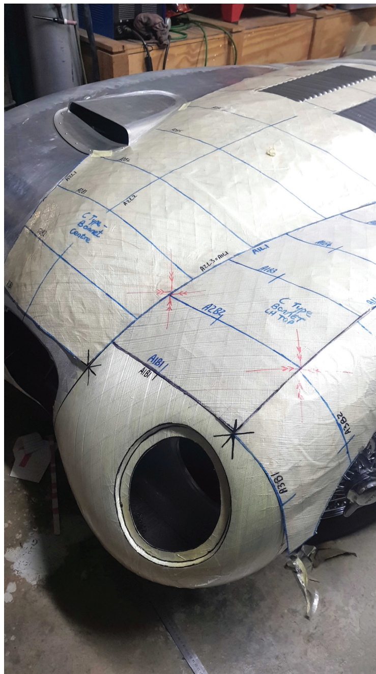
Detailed mapping of his father's aluminium C-Type. Soon Conrad will be building his own.
