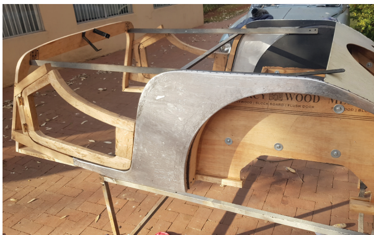
Conrad's Morgan Plus 8 for which he had to rebuild the oak wood frame and aluminium body work due to fire damage.
