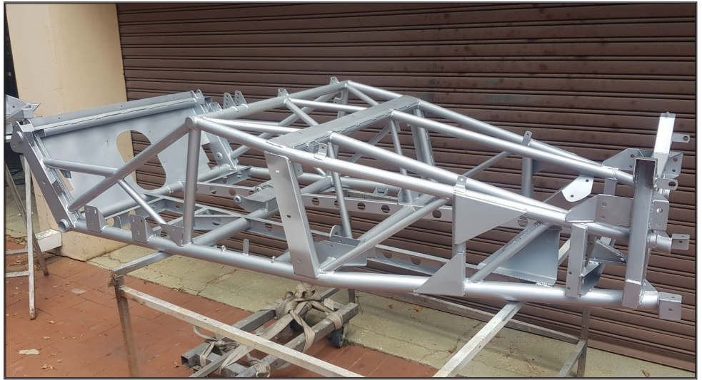
One of two C-Type chassis made by Conrad by reverse engineering. Conrad built one for himself and the other for his father..
