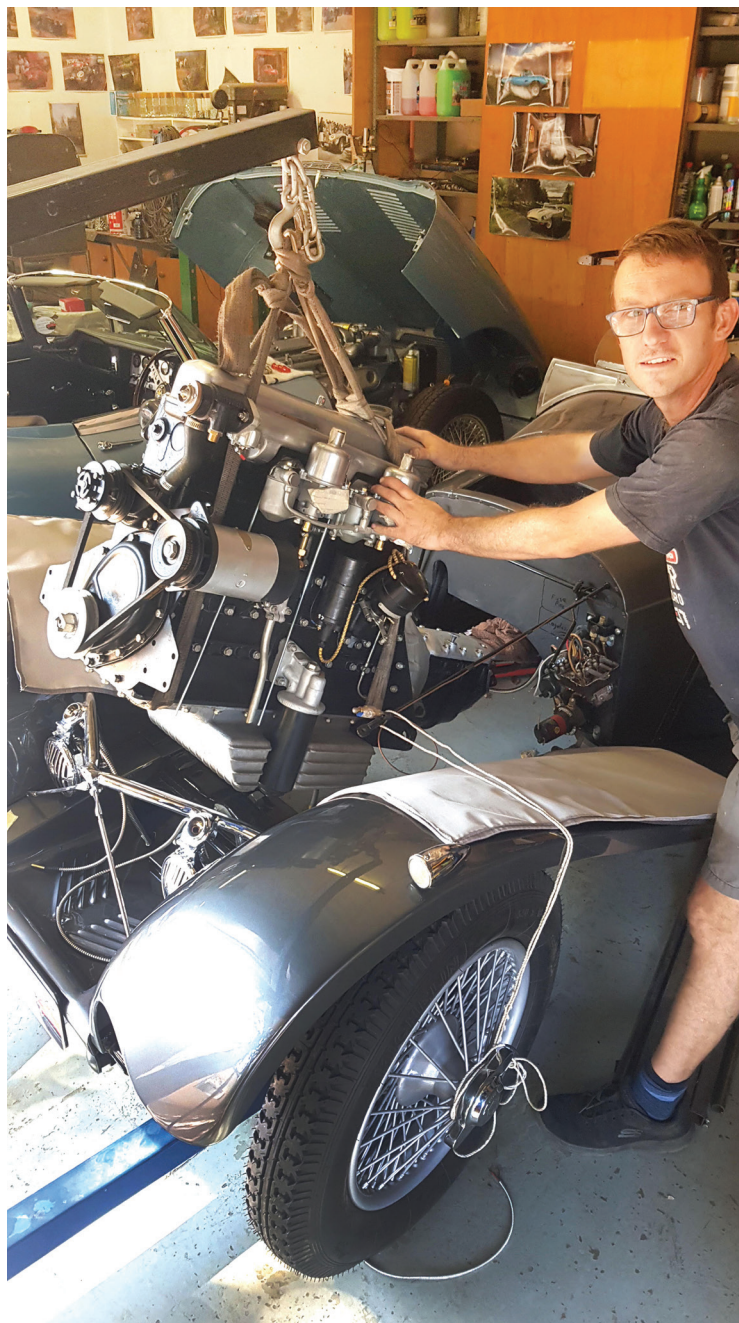
Replica SS100: Engine & gearbox assembly being fitted to the car.
