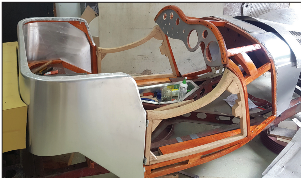
Replica SS100: Progress of new wood frame and aluminium body work. (Built for a client).
