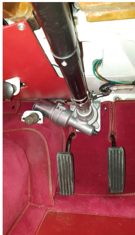
Column installed in XK140
