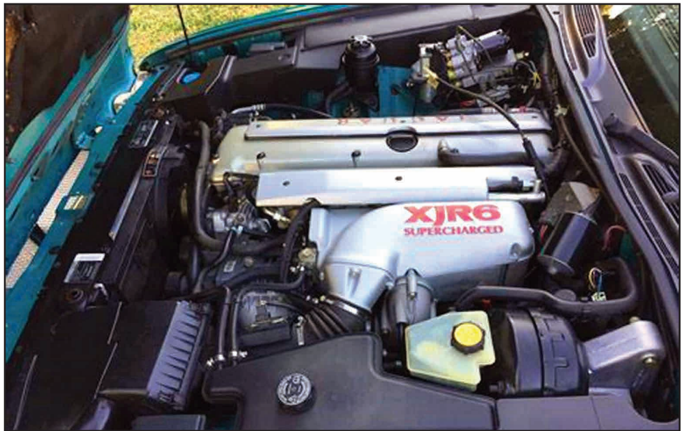
1995 XJR supercharged AJ16 engine producing 326 hp (243 kW; 331 PS) and 378 lb-ft (512 N-m) with the use of an Eaton M90 supercharger and an air-water intercooler.
