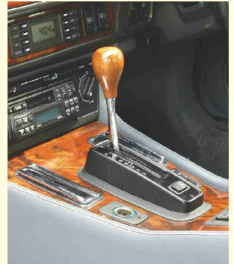
When the V12 XJ-S became a 6.0-litre in 1993, the gearbox was also upgraded to a four-speed unit.
