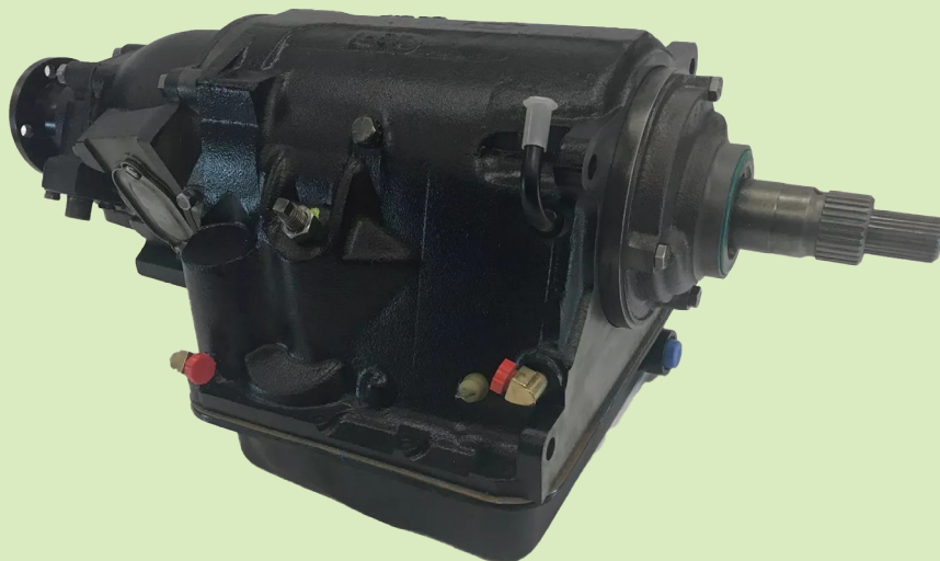
From launch until 1977, if you specified an automatic V12 XJ-S, then it came with the three-speed Borg Warner Model 12.
