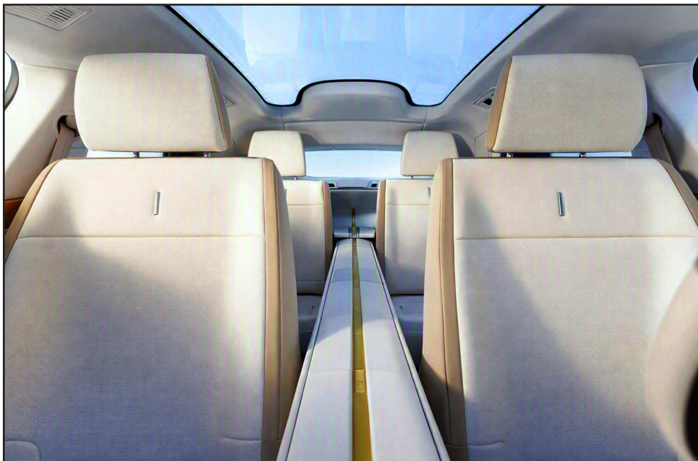
The Jaguar Type 01 features minimalist seats front and rear, a strong brass-trimmed centre spine, a long panoramic glass roof and no rear window. (Jaguar media).
