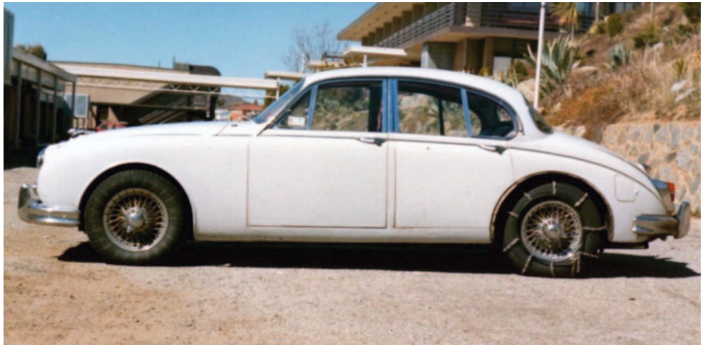
Snow chains fitted to the rear drive wheels
