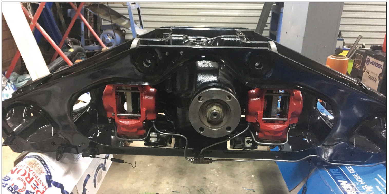
Completed rebuilt rear independent suspension and differential.
