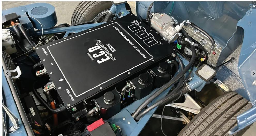
the motor and running gear route their way back through the chassis. ECD claims its electric E-Type can do about 200 miles of city driving or 140 miles of highway driving.
