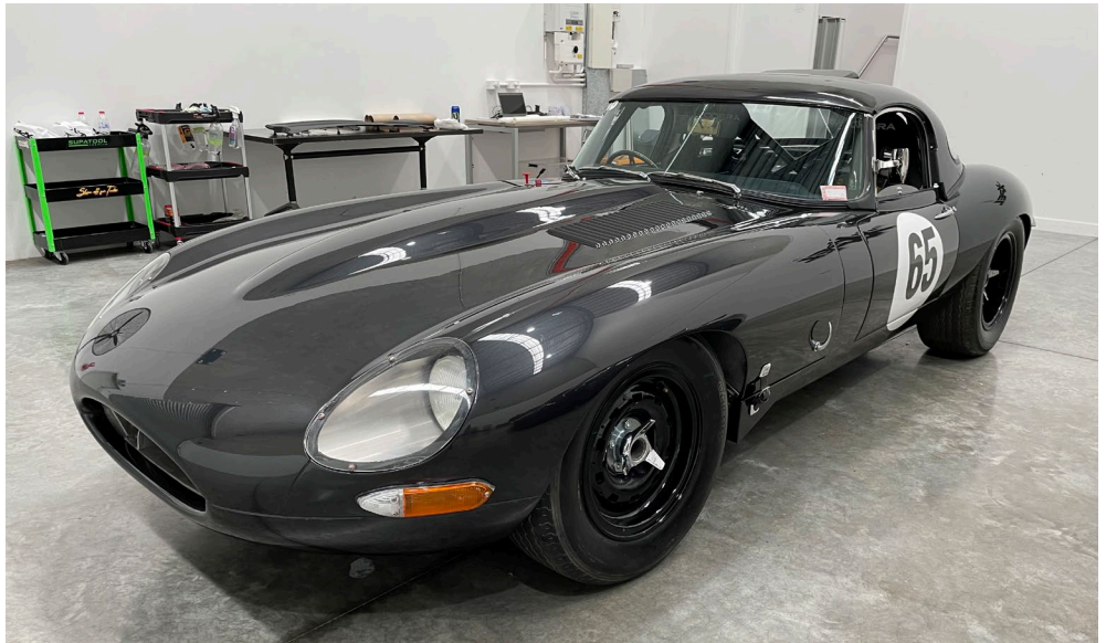
Car No. 3. Phil's FiA compliant LWT race car complete with purpose built fuel injected Crosthwaite & Gardiner (UK) aluminium block and wide angle head.
